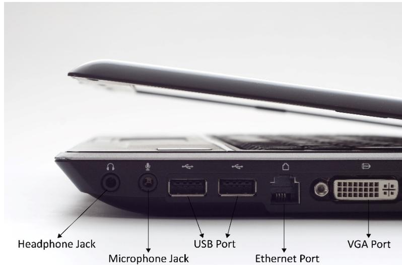
*Fig. 4.1.11: Different connection ports in a laptop computer*
