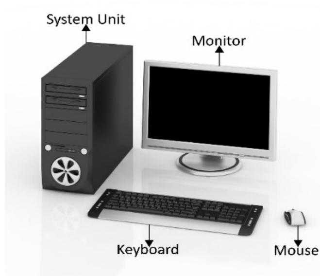
*Fig. 1.1.16: A desktop computer along with its CPU and peripherals*
