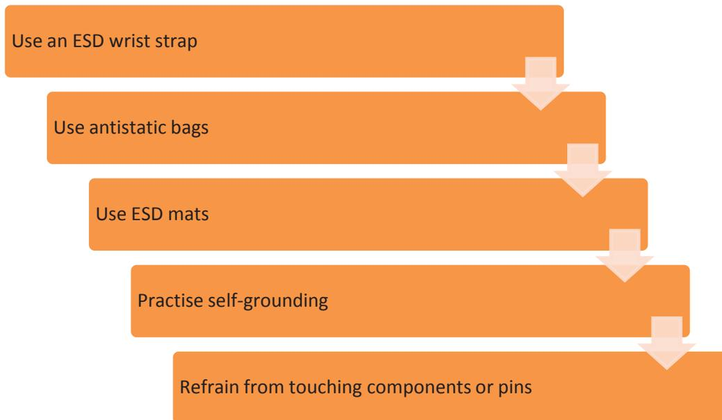
*Fig. 1.3.6: Steps to be taken for ESD damage reduction*
